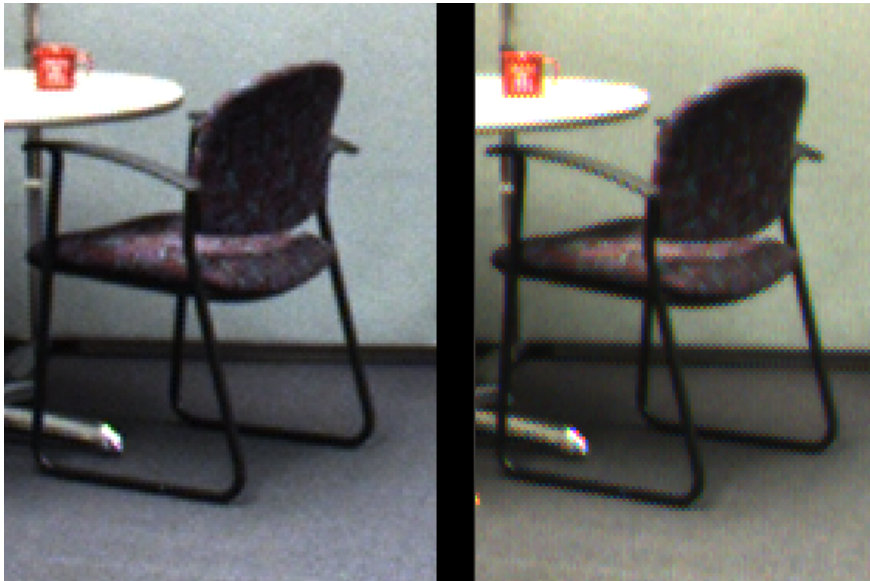
Figure A.3: An advanced demosaicing method (HQLinear (Malvar et al., 2004)) and a quick, but less accurate demosaicing method (Nearest Neighbour)
