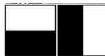
Figure 3.5: The Haar wavelets that are used in SURF to calculate the orientation of the interest points. Image from Bay et al. (2006)
